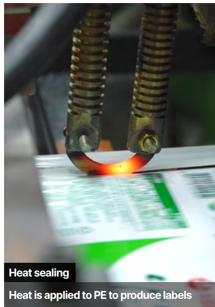
Sealing/inspection Produce and inspect shrink labels by sealing into tubes
